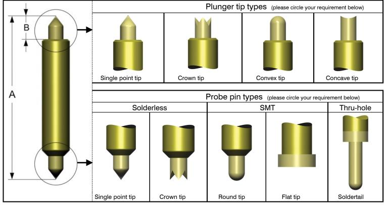
Probe pin and Connectors are generally produced to custom specifications.
